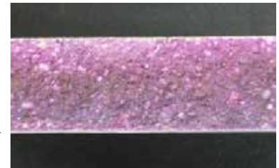
RIGHT: No penetration of carbonate with ecotio 2 ® as the indicator is unaffected →
