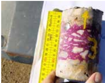
← LEFT: Unprotected concrete showing where the purple indicator has changed colour to white due to carbonation
